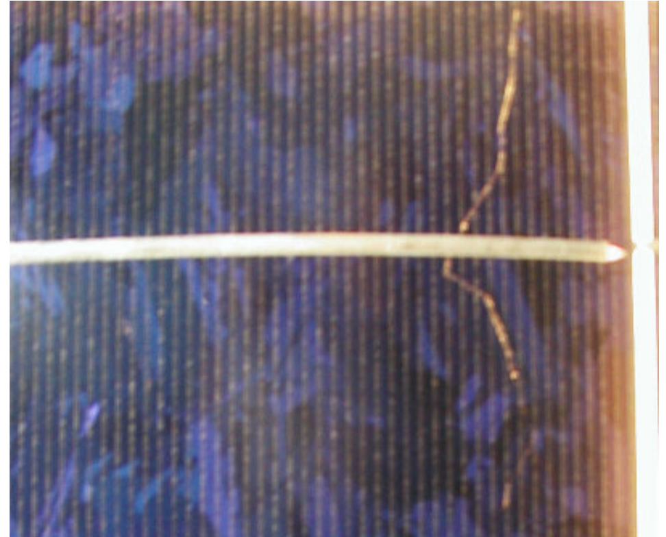
Cracking of solar cells
