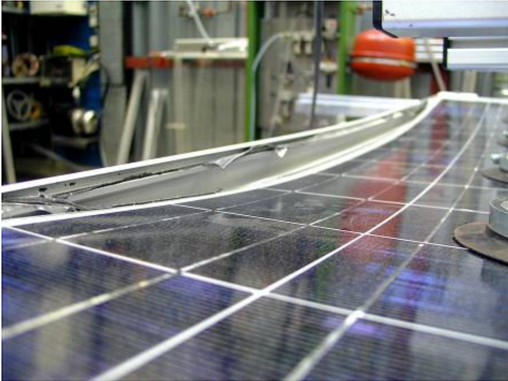
Insufficient stability of frame
